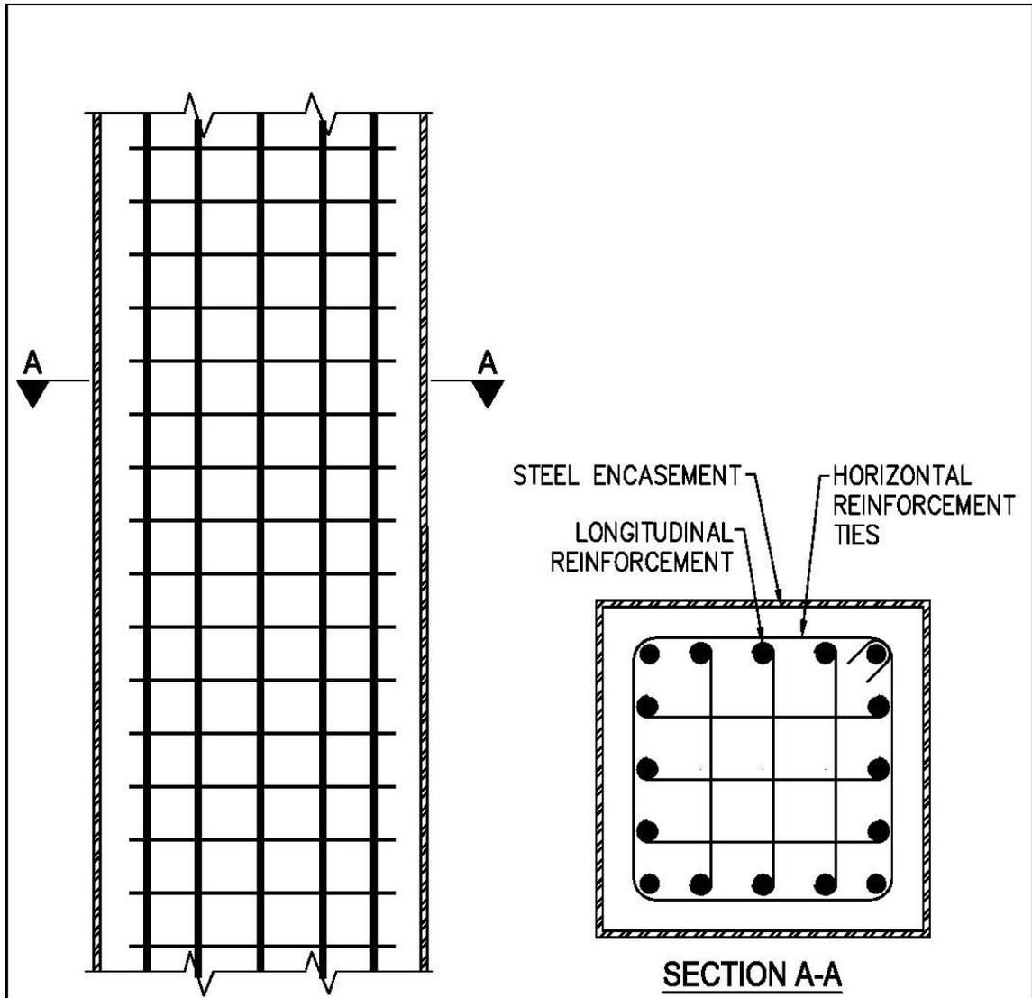
**10B CONCRETE COLUMN WITH STEEL JACKET DETAIL-1**
