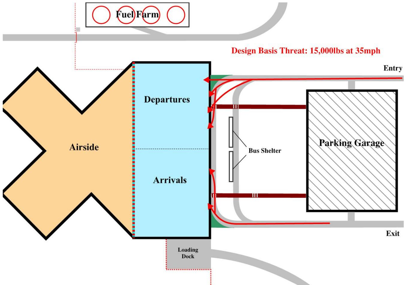
Shallow mounted bollards have been selected due to the presence of underground services beneath the footpath outside the entrances to the airport. These foundations (depth less than 12 inches) can sit atop these services.
