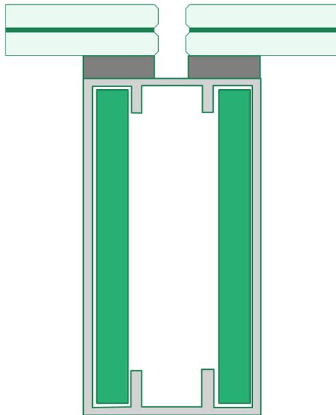
Figure 4-14. Framing Split-Section with a Blast Clip
