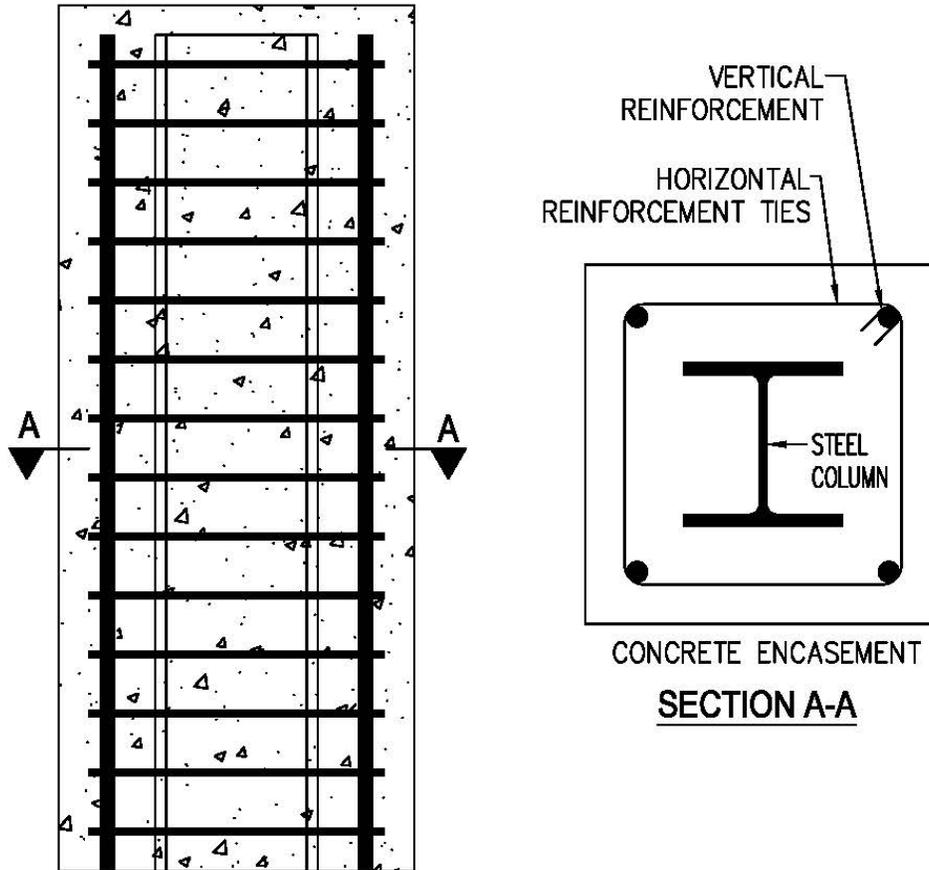
**7 ENHANCED COLUMN - CONCRETE ENCASEMENT**
