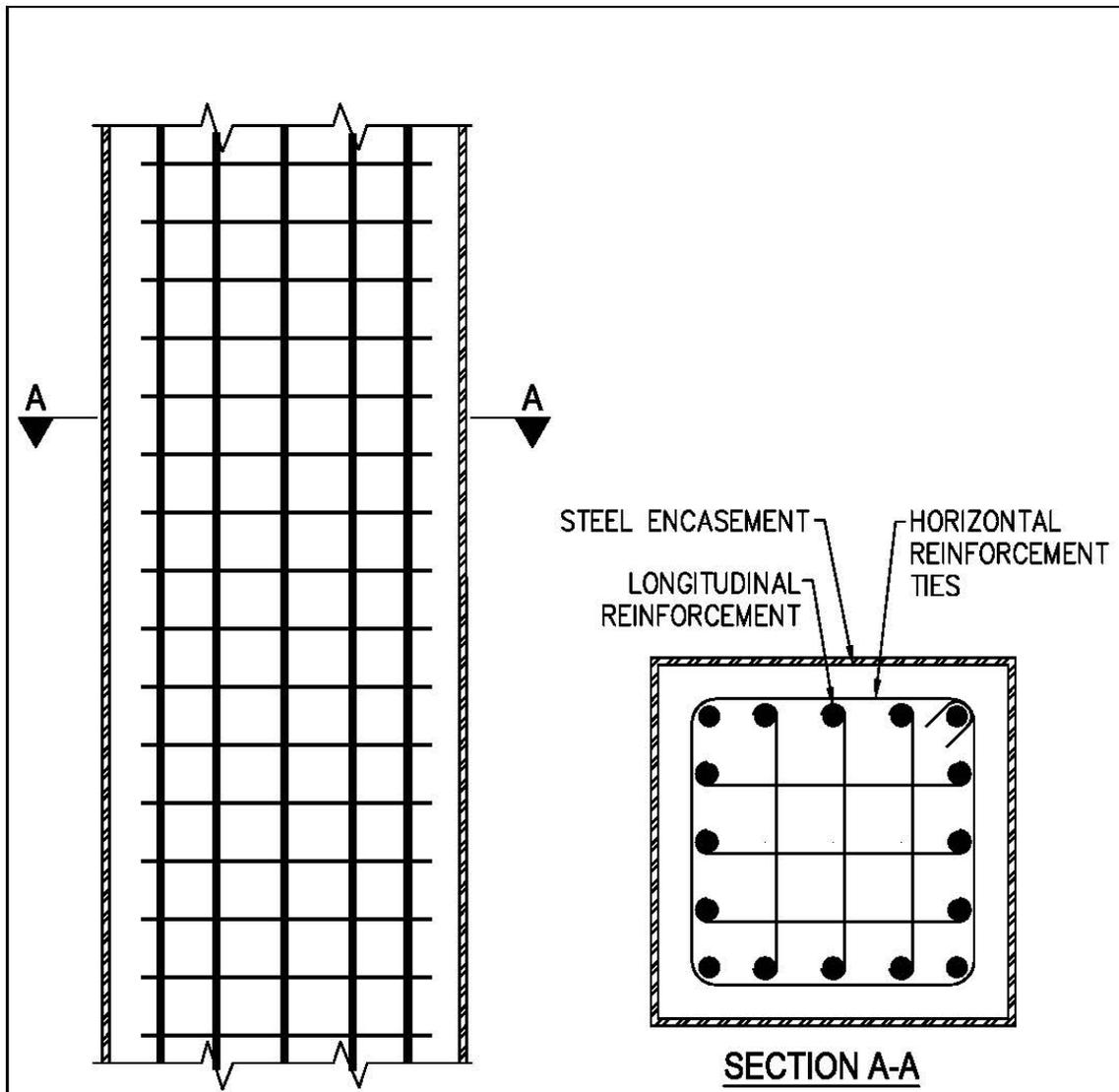
**10B CONCRETE COLUMN WITH STEEL JACKET DETAIL-1**
