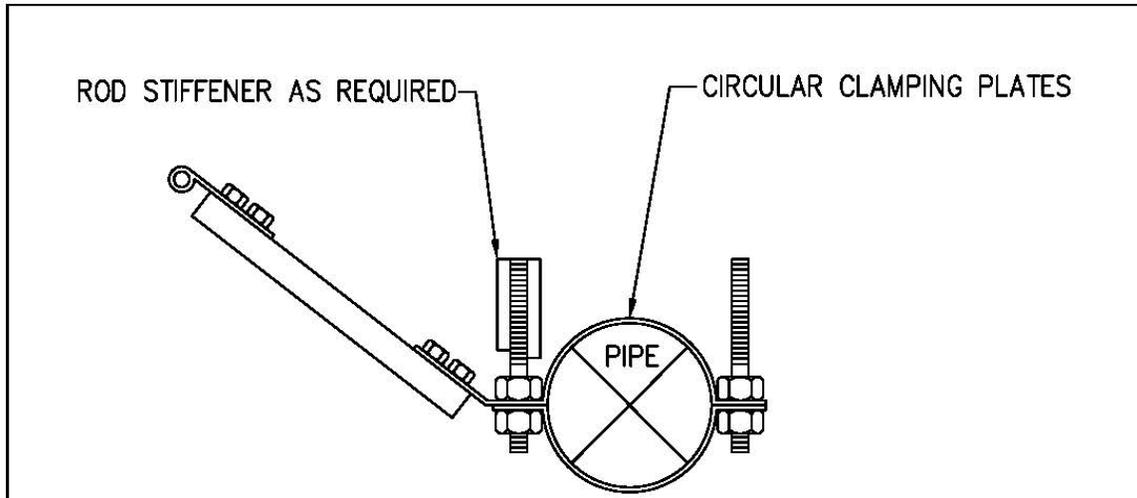
**21 RESTRAINT OF PIPEWORK WITH U-BOLT**
