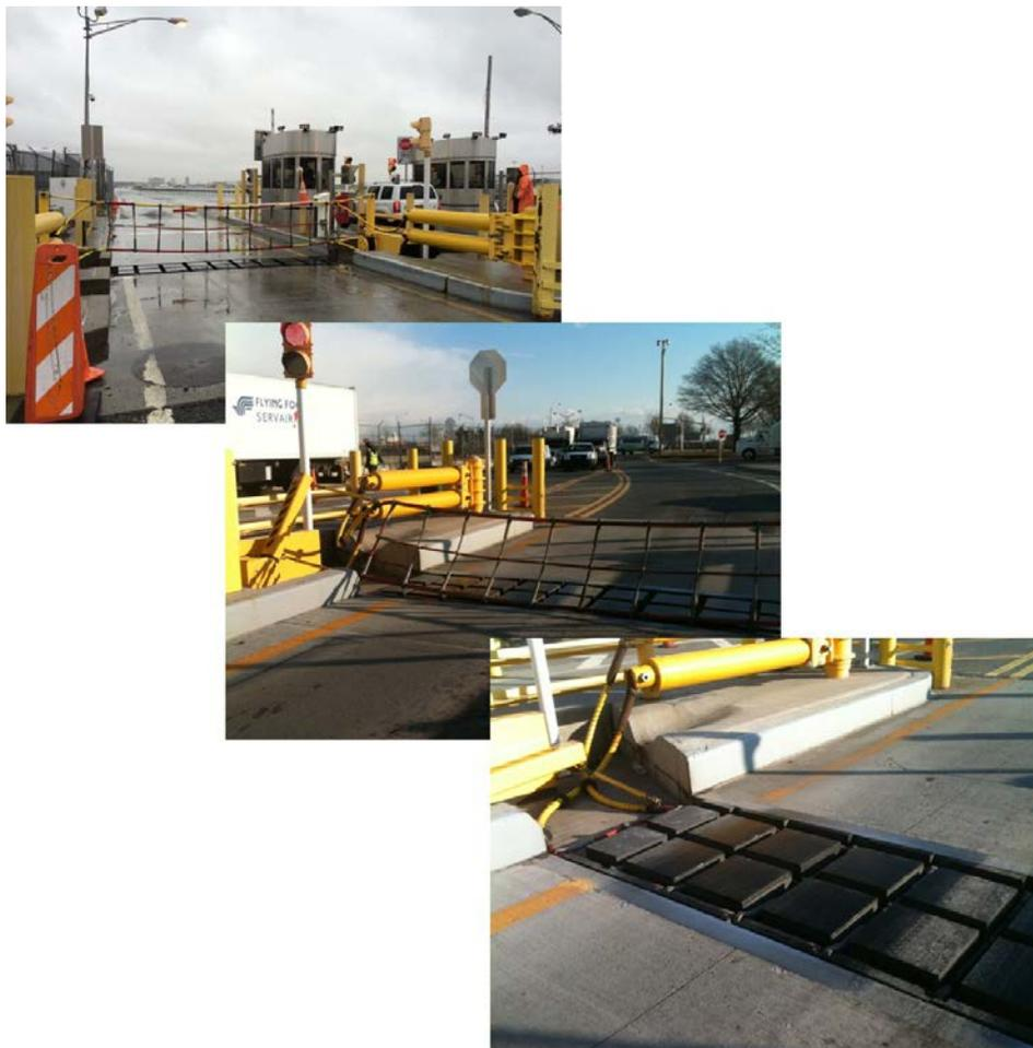
The photographs show the net fully engaged (top), as it drops (center), and finally as it is fully disengaged to allow vehicle passage (bottom).
